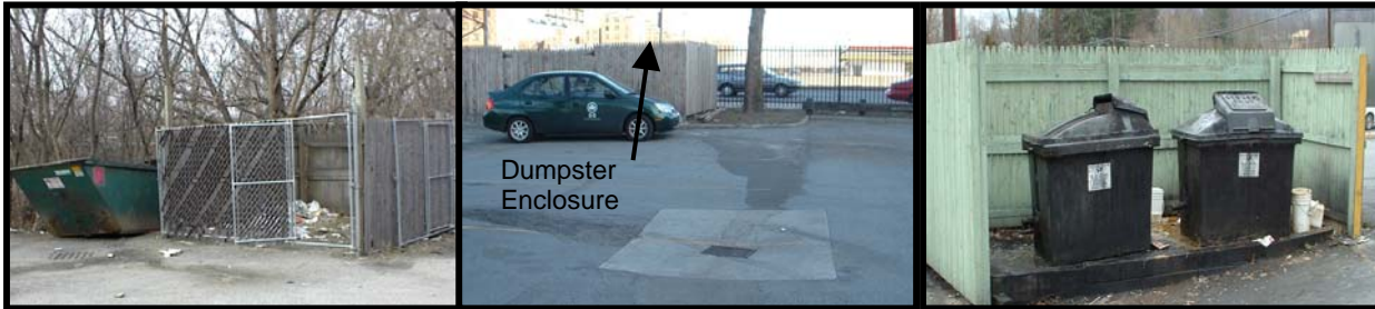
Typical signs of poor dumpster management: trash accumulation and uncovered dumpster near storm drain
