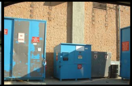
Materials are covered to prevent pollution of stormwater
